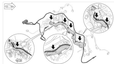
Laying line for exhaust temperature sensor
