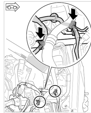
Clipping in wire harness on the fuel gallery
