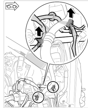
Unclipping wire harness
